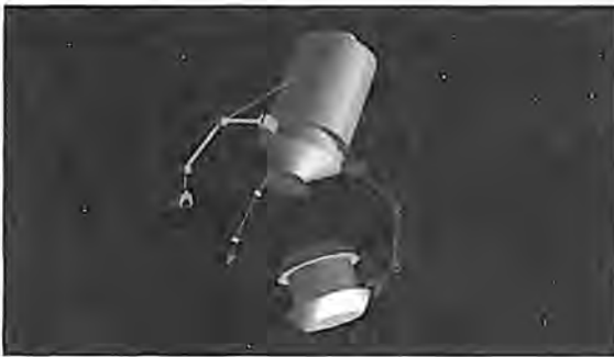
FIGURE P8.20 A space robot with three arms, shown capturing a satellite.
